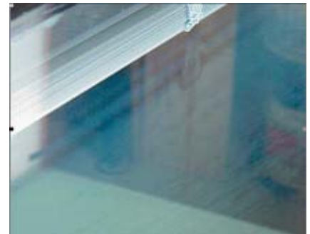
Figure 2 Whitish contamination on the second glass surface caused by corrosion of the surface
